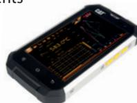
When connected to a Cyclops pyrometer, the Logger software records instantaneous temperature measurements each time the pyrometer trigger is pressed.
